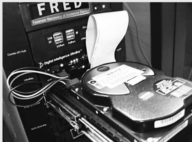
A hard disk is imaged using one of BEAM's "capture" workstations.
