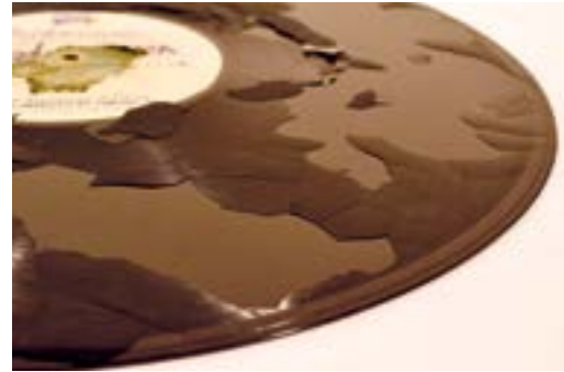
Laminate separation on a glass-based lacquer disc
