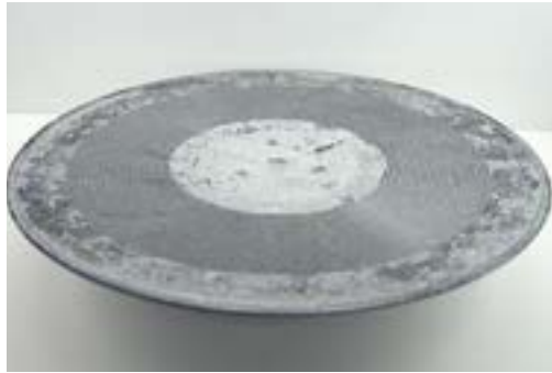
Palmitic acid exudation on a lacquer disc
