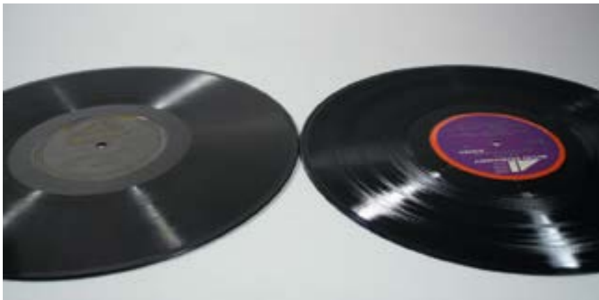
A side-by-side comparison of a 12-inch 78-rpm disc and a 12-inch LP shows the matte surface of shellac and the reflectivity of vinyl discs.
