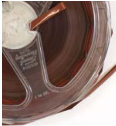
Tight Spoking, cupping/curling
