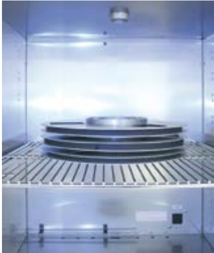
Tapes being baked in an industrial oven. Note use of tape hub spacers between stacked reels.
