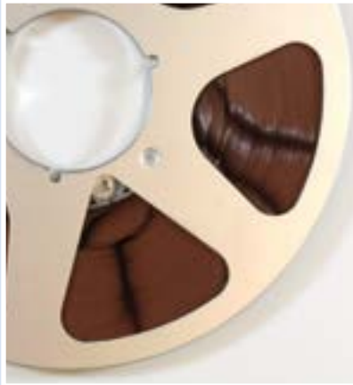
Loose Cinching, windowing
